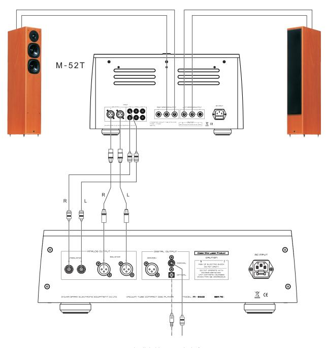
To the digital input terminal of a D/A converter or digital amplifier
