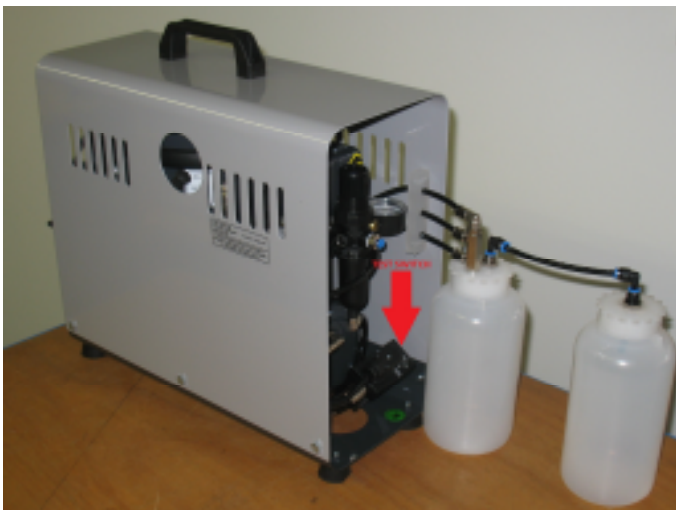
Fig. 3. Compressor with “Double PVC drain bottles”
