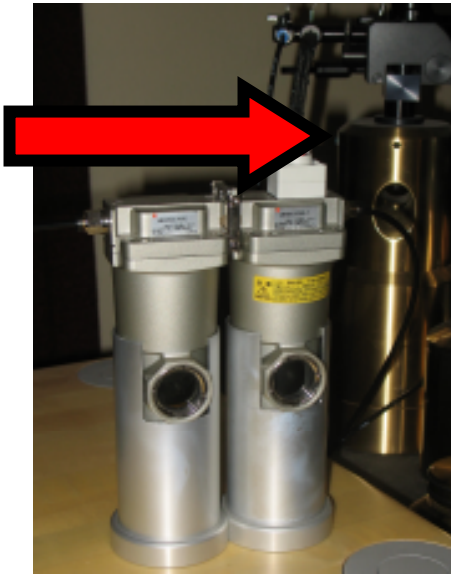
Fig. 7. Silver filters- see arrow for airflow
