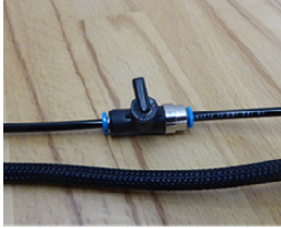
Fig. 9. Valve in closed position
