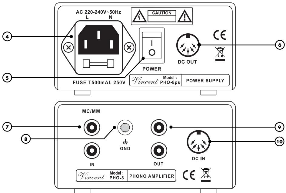
**4. AC/FUSE: power connector and fuse holder**
