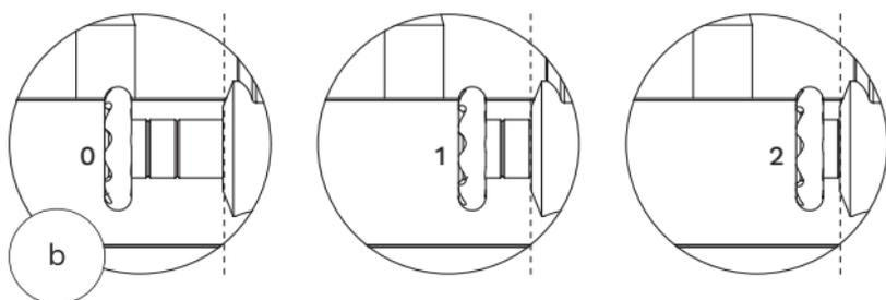
Simply push the bias adjustment slider in to the required setting, using the dotted line as your reference (**as shown above**).
