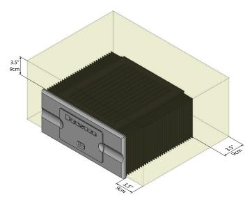
Minimum recommended clearance for heat dissipation
